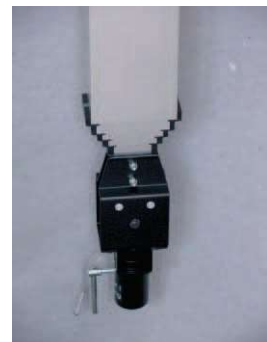
Load attachment through DIN socket (Ø 29 mm)
